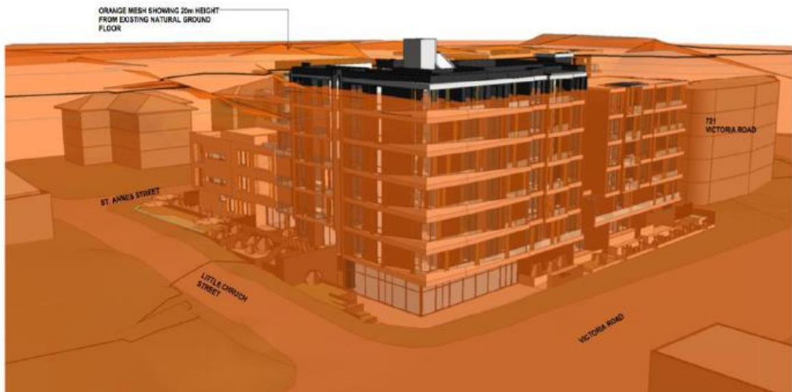
Figure 20: Extent of height breach
